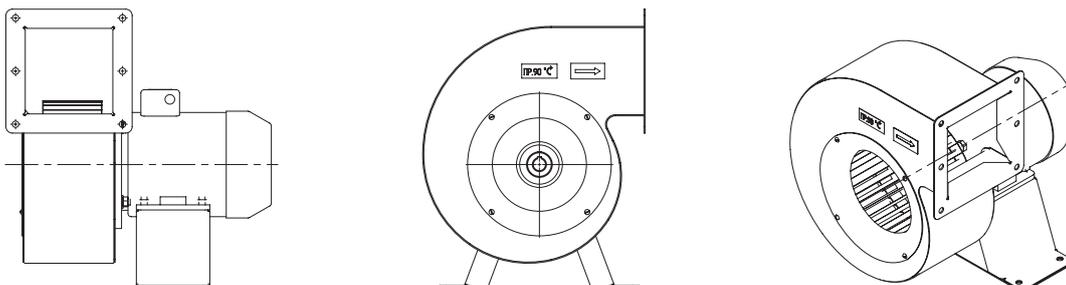
VCUN modifications must be agreed in the orders (body position, direction of rotation of a turbine, protective grille, round duct, motor base vibration insulation).
